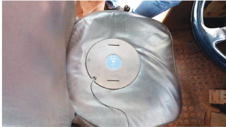
Figure : 1 A tri-axial seat-pad accelerometer placed on the seat of the operator
