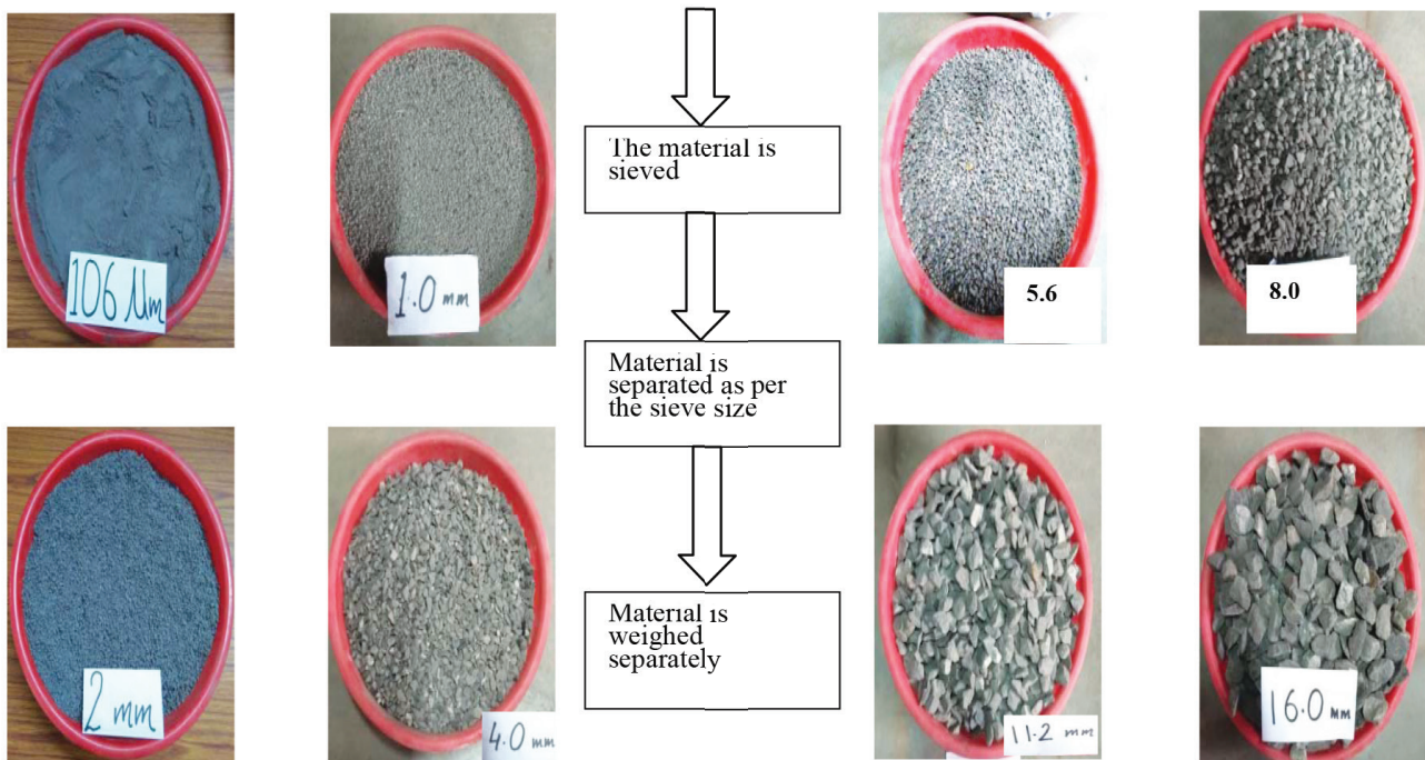
Figure 1. Different sizes of the material mix used for after sieving obtained from overburden dump
