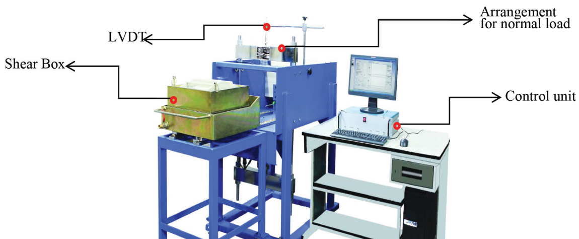
Figure 2. Direct shear testing setup of 30 cm X 30 cm shear box size
