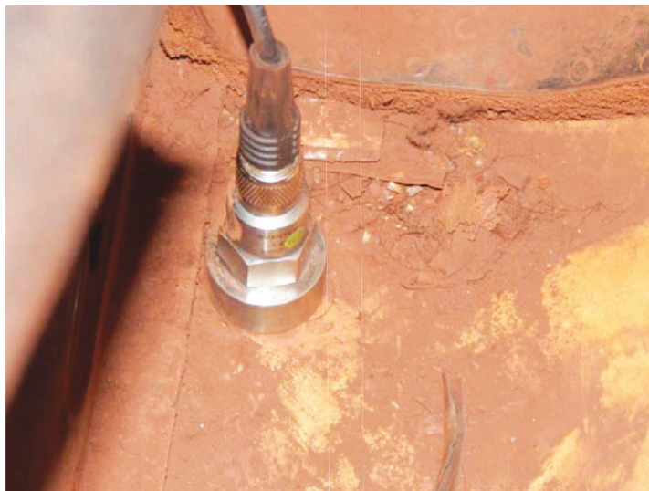
Fig 2 : SV80 mono-axial accelerometer magnetically secured to the floor of the driver's cabin
