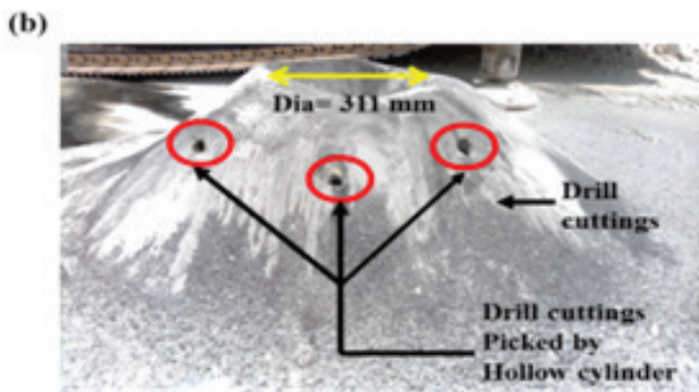
Fig.2 (b) Method of drill cuttings collection
