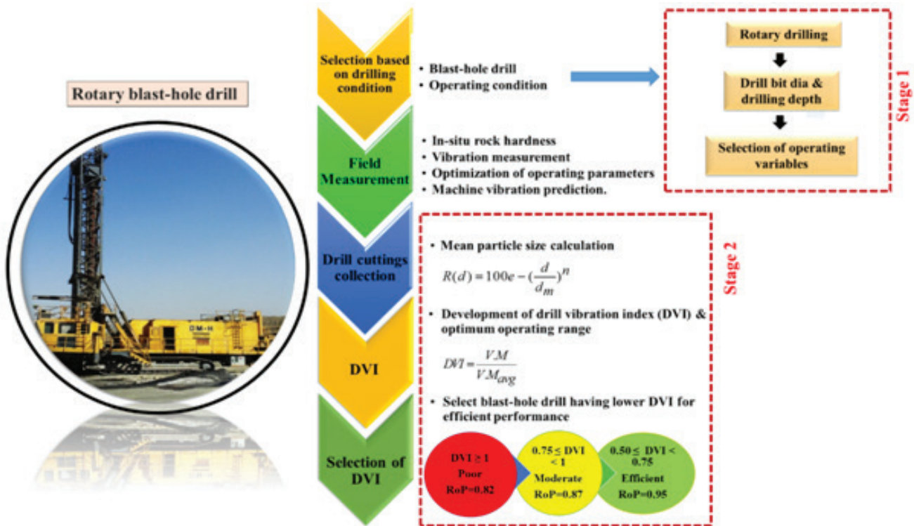
Fig 11. Rotary blast-hole drill operational strategy
